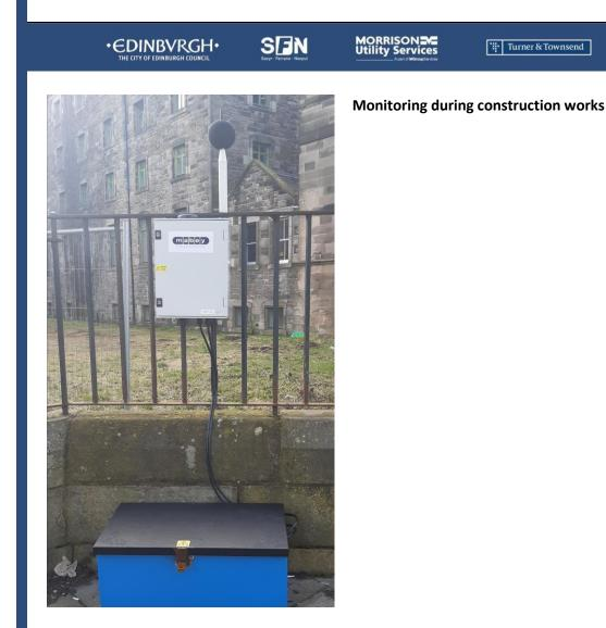
During the construction works we are required to monitor noise and vibration levels. In order to achieve this there have been six noise and vibration monitoring systems installed across the route to ensure that we are monitoring any associated noise and that we do not exceed the agreed limits.
