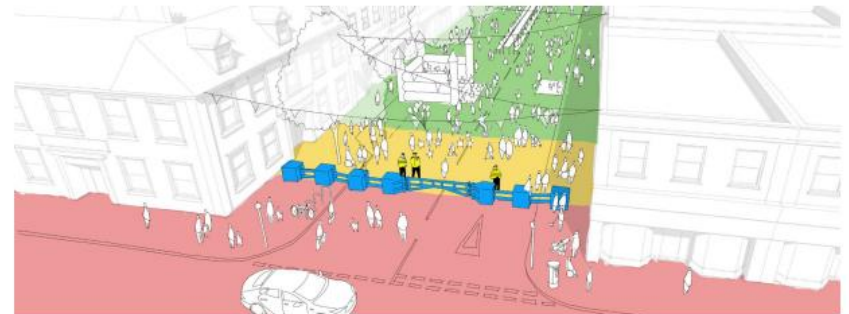
(c) Temporary protection - Temporary or redeployable Vehicle Security Barriers (VSBs) may be employed at times of heightened threat or pre-planned special events. These barriers require specialist equipment to deploy, tend to be more visually intrusive and less permeable for pedestrians than permanent solutions.
