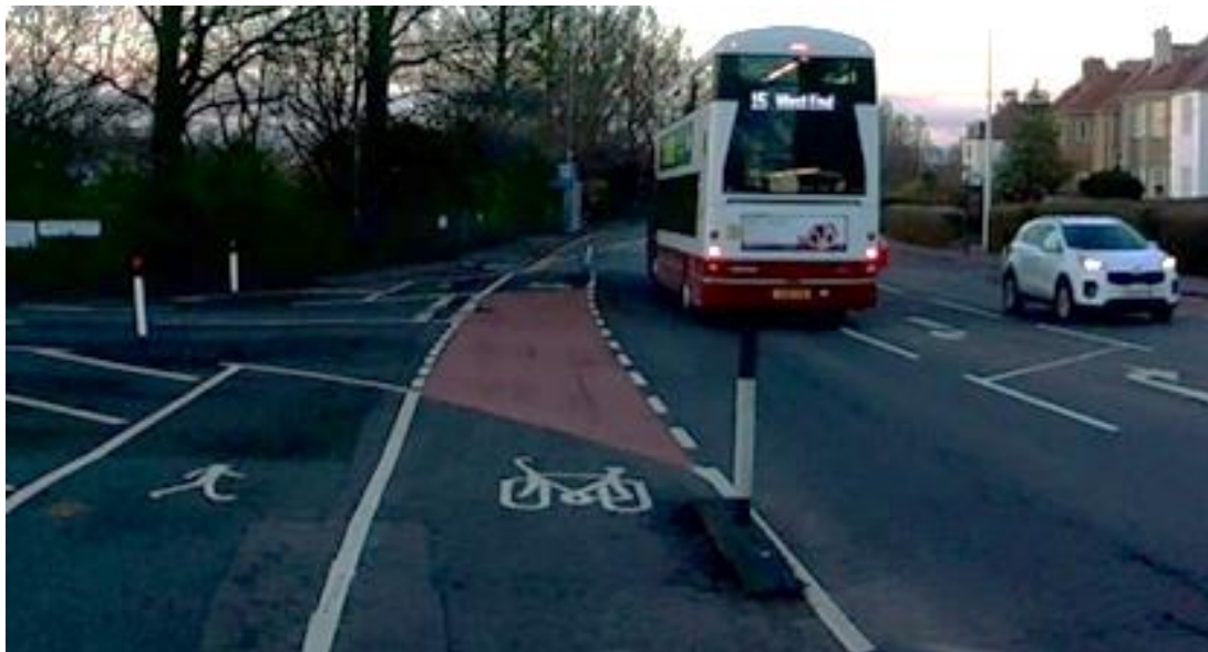
Figure 3-1: Lane Defenders Reduce Turning Radii
