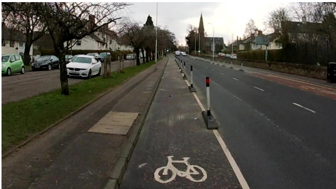
Figure 2-1: Example of a Segregated Cycle Lane with Lane Defenders on Gilmerton Road
