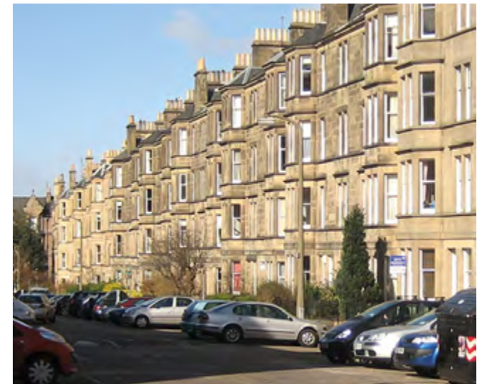
Generous window heights: Marchmont, Arden Street - These tenements manage to provide good levels of daylight to all the properties. This is a result of the high floor to ceiling heights and relatively large and tall windows which allow daylight to go deep into the rooms.
