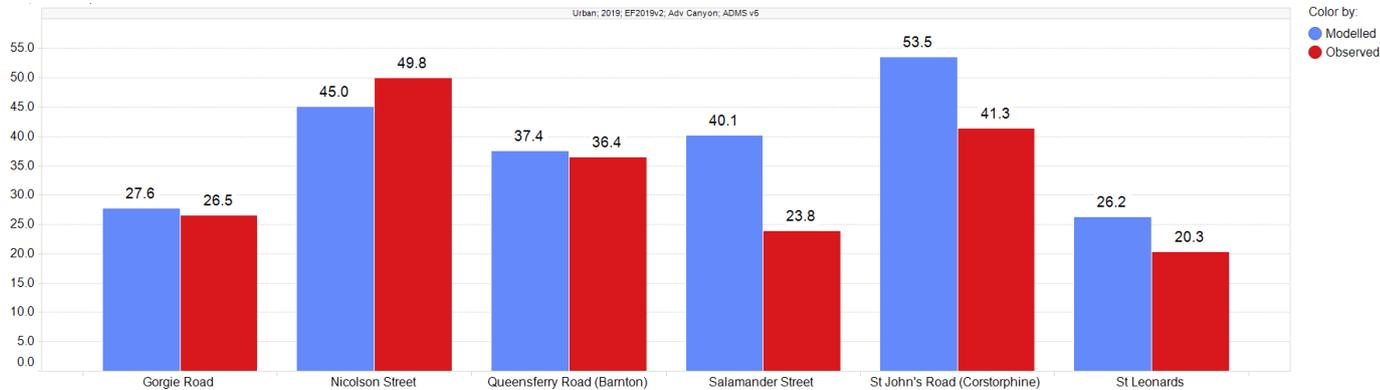
Figure 86: Modelled and Measured 2019 NO<sub>2</sub> Concentrations at Automatic Monitors (ADMS-Urban 5.0)
