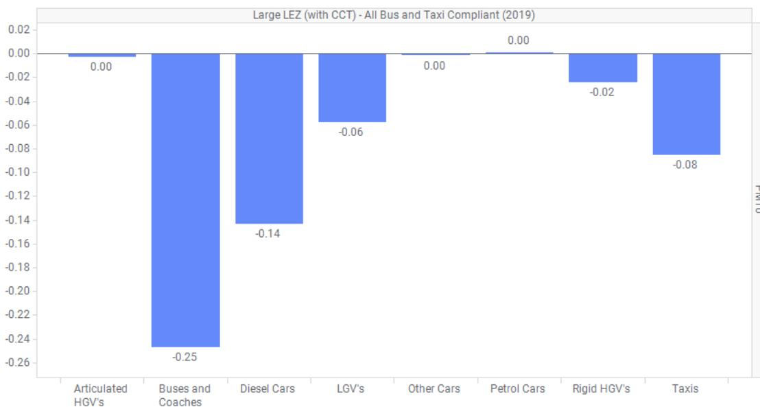
Figure 38: Changes in PM<sub>10</sub> Emissions (Large LEZ option) from each vehicle sector for within the LEZ when compared to Base 2019 scenario (tonnes/yr)
