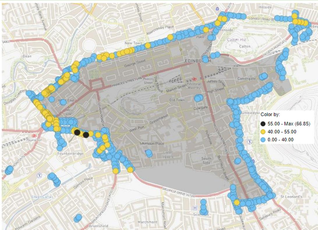
Figure 76: Predicted NO<sub>2</sub> concentrations ( $\mu\text{g m}^{-3}$ ) at façade receptors (Large LEZ 2019)
