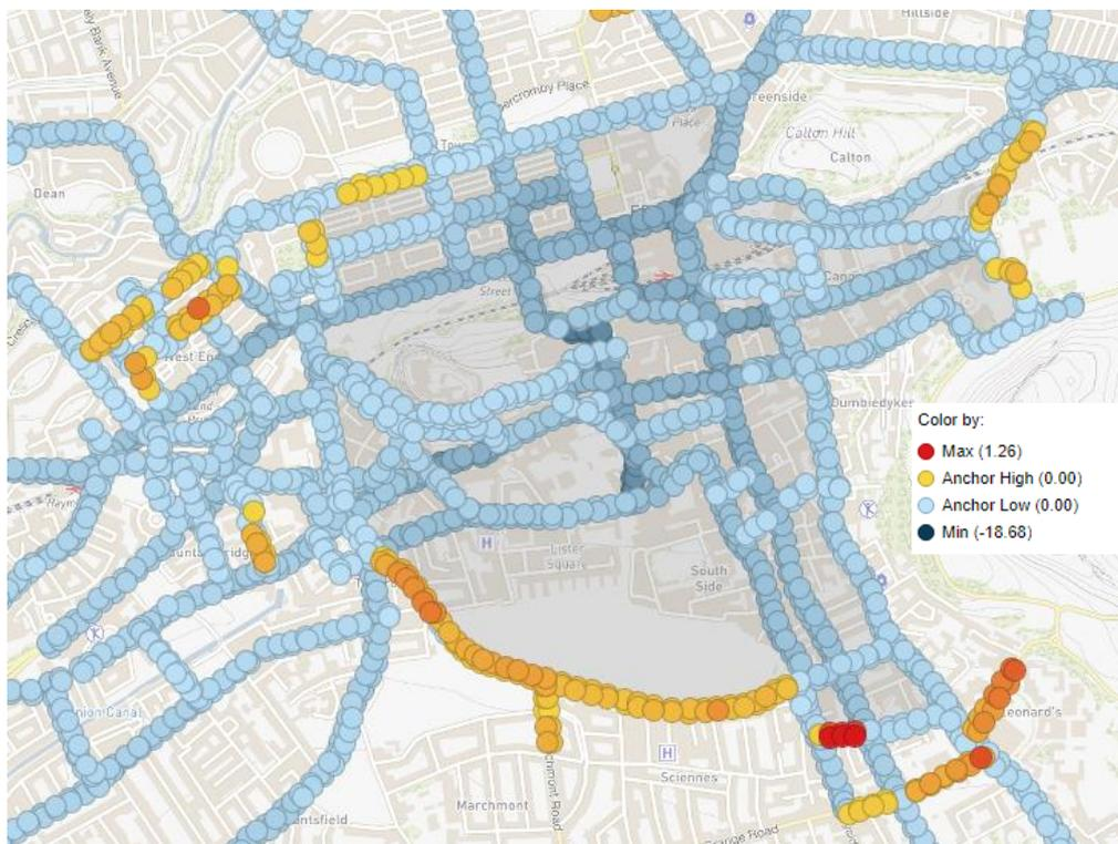
Figure 63: Predicted Changes in  $\text{NO}_2$  concentration ( $\mu\text{g m}^{-3}$ ) due to introduction of Small LEZ (2023), when compared to 2023 Base scenario
