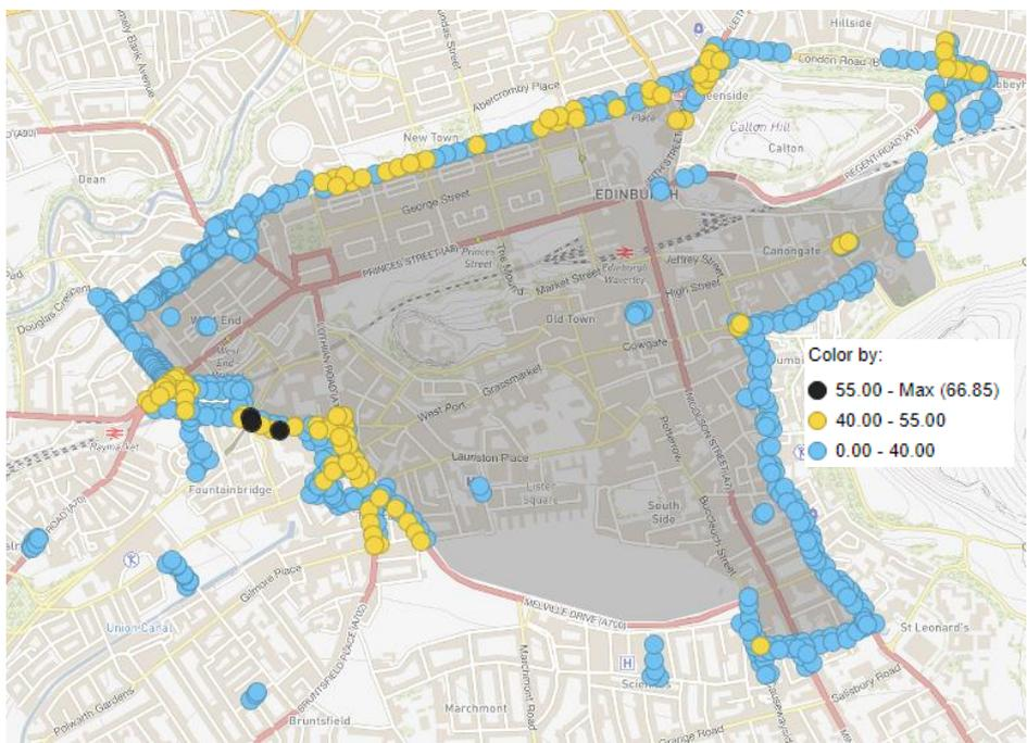
Figure 75: Predicted NO<sub>2</sub> concentrations (µg m<sup>-3</sup>) at façade receptors (Base 2019)
