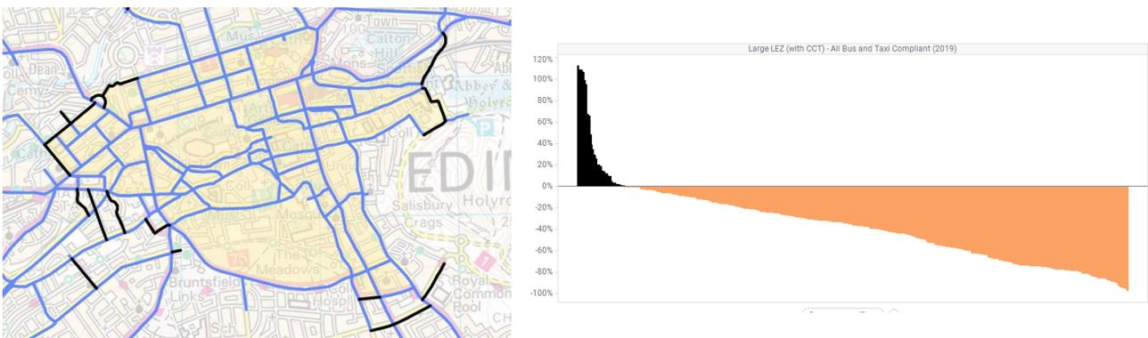
Figure 27: Relative changes to PM<sub>10</sub> emissions when comparing the Base 2019 scenario and Large LEZ 2019 option. Street highlighted are those where an increase in emissions is predicted
