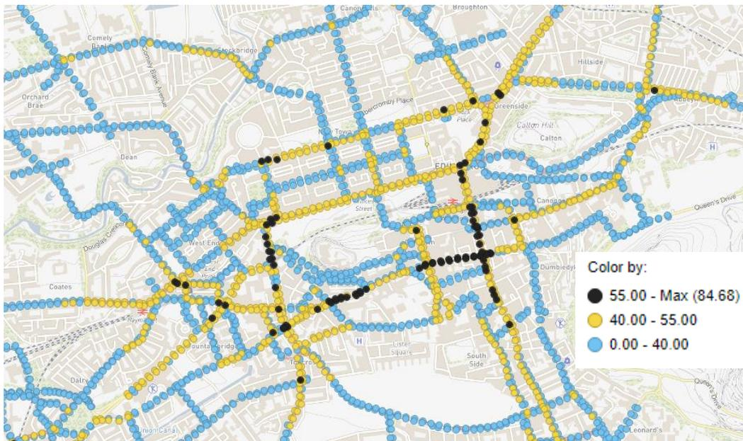
Figure 41: **Base** 2019 NO<sub>2</sub> predicted concentrations ( $\mu\text{g m}^{-3}$ )
