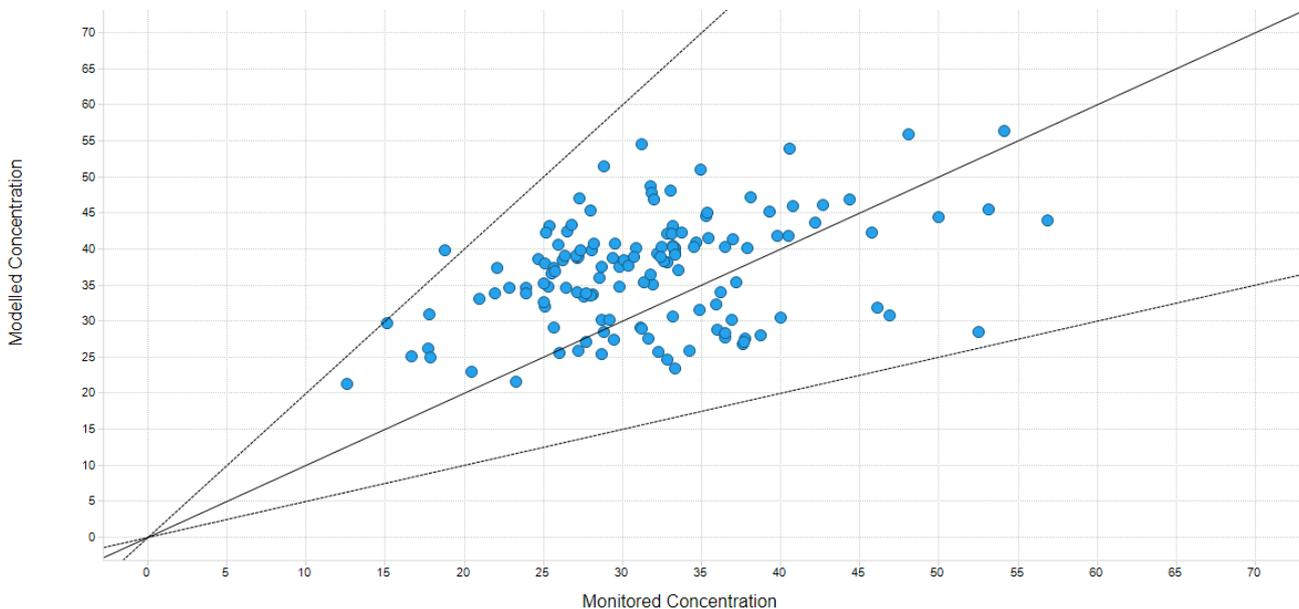
Figure 87: Modelled v Monitored NO<sub>2</sub> Concentration Scatter Plot for Diffusion Tube Locations for 2019 (ADMS v5; Urban Background; Bias-adjusted diffusion tube data)
