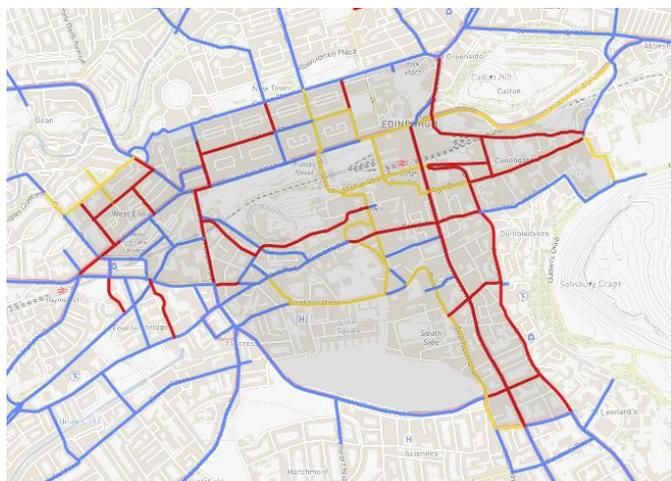
Figure 90: Total Petrol Car Traffic Flow Relative Differences (2019) for Large LEZ option, when compared to Base scenario
