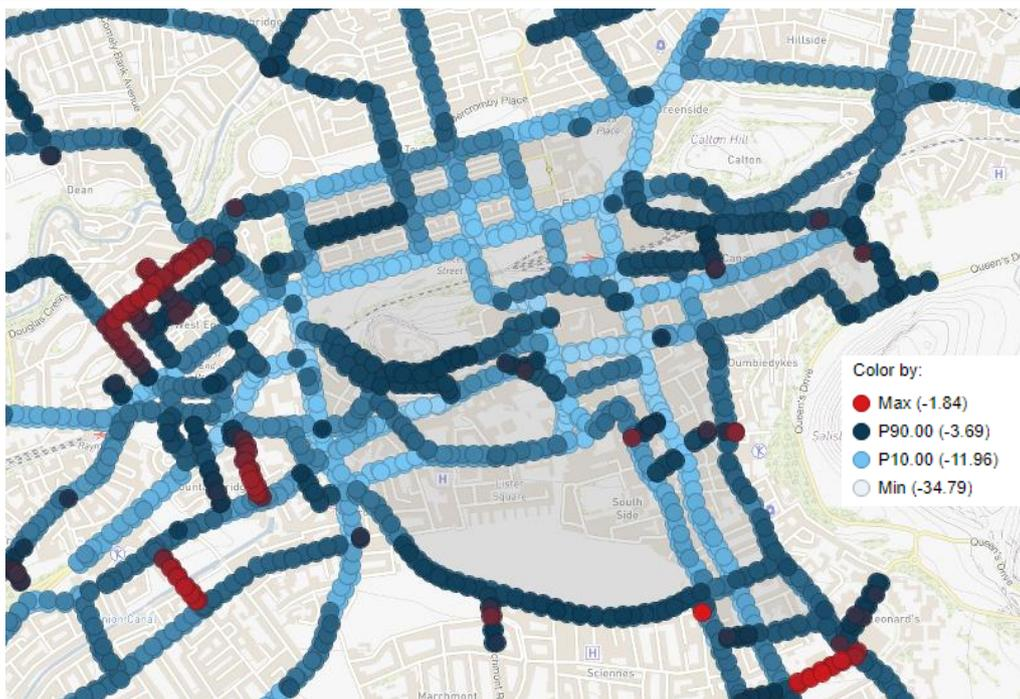
Figure 60: Predicted Changes in NO<sub>2</sub> concentration ( $\mu\text{g m}^{-3}$ ) due to Large LEZ (2023), when compared to 2019 Base scenario
