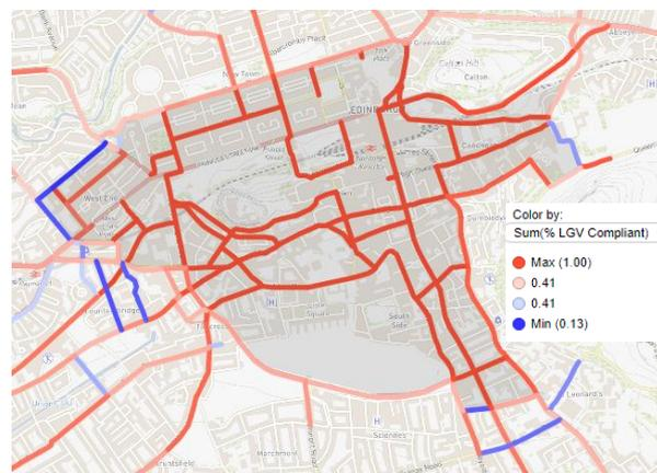
Figure 94: Compliance % of LGV's on each road link for the Large LEZ option (2019). 41% is the 2019 compliance value for LGV's
