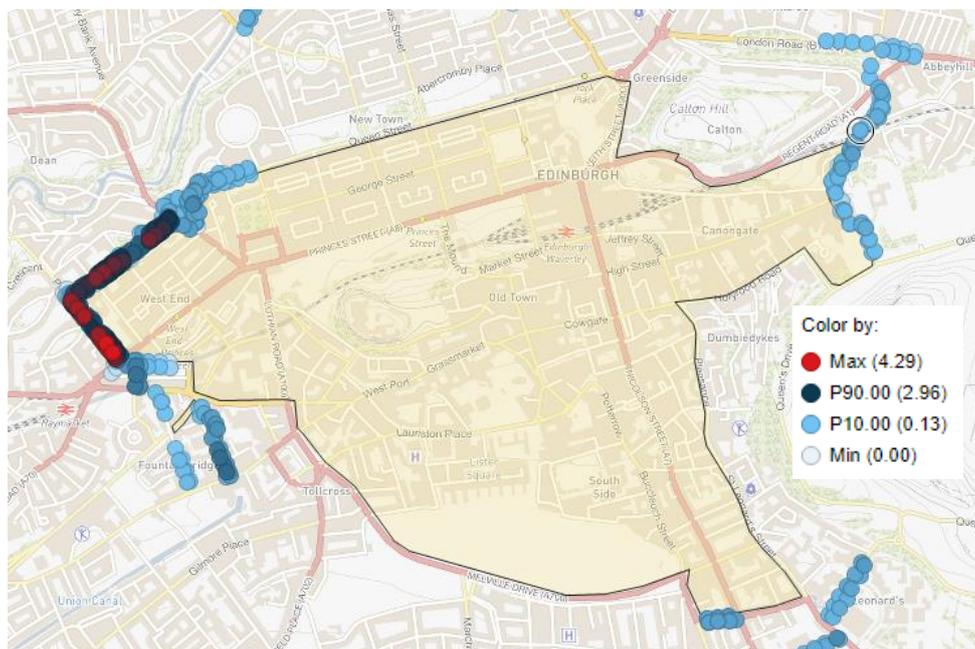
Figure 61: Predicted NO<sub>2</sub> increases ( $\mu\text{g m}^{-3}$ ) due to Large LEZ (2023), when compared to 2023 Base scenario
