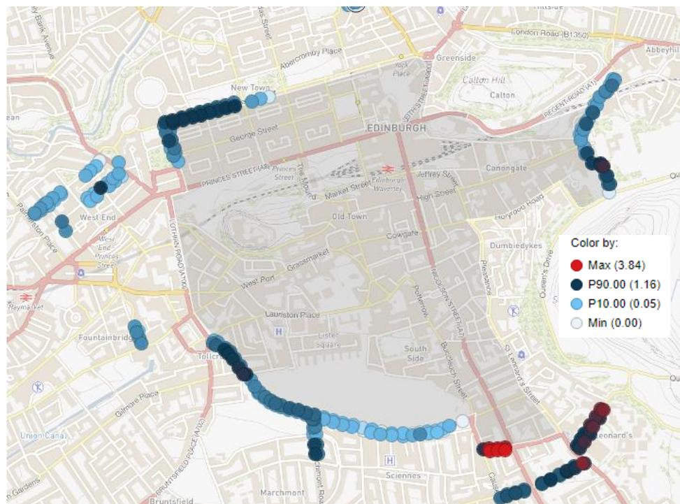
Figure 51: Predicted NO<sub>2</sub> increases (µg m<sup>-3</sup>) due to introduction of Small LEZ (2019), when compared to 2019 Base scenario
