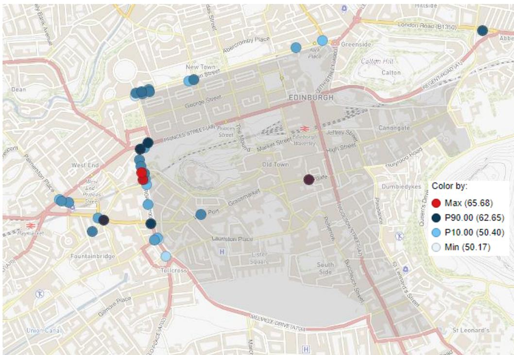
Figure 53: Predicted NO<sub>2</sub> concentrations  $>50 \mu\text{g m}^{-3}$  due to introduction of Small LEZ (2019)
