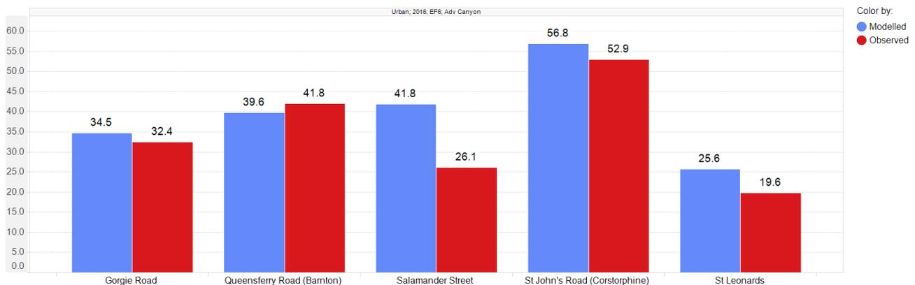
Figure 83: Modelled and Measured 2016 NO<sub>2</sub> Concentrations at Automatic Monitors (ADMS-Urban 4.2)
