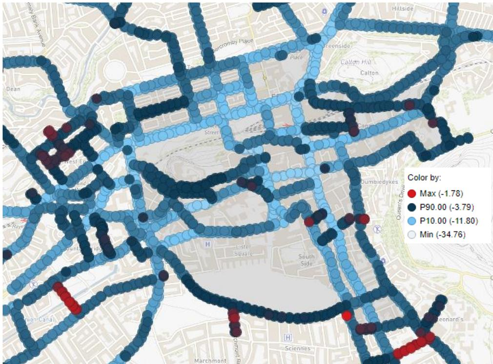
Figure 65: Predicted Changes in NO<sub>2</sub> concentration ( $\mu\text{g m}^{-3}$ ) due to introduction of Large LEZ (2023), when compared to Base 2019 scenario
