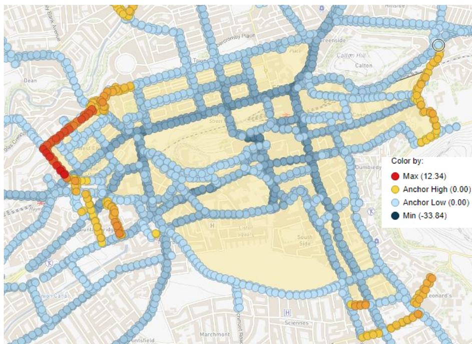
Figure 44: Predicted Changes in NO<sub>2</sub> concentration (µg m<sup>-3</sup>) due to introduction of Large LEZ (2019), when compared to 2019 Base scenario
