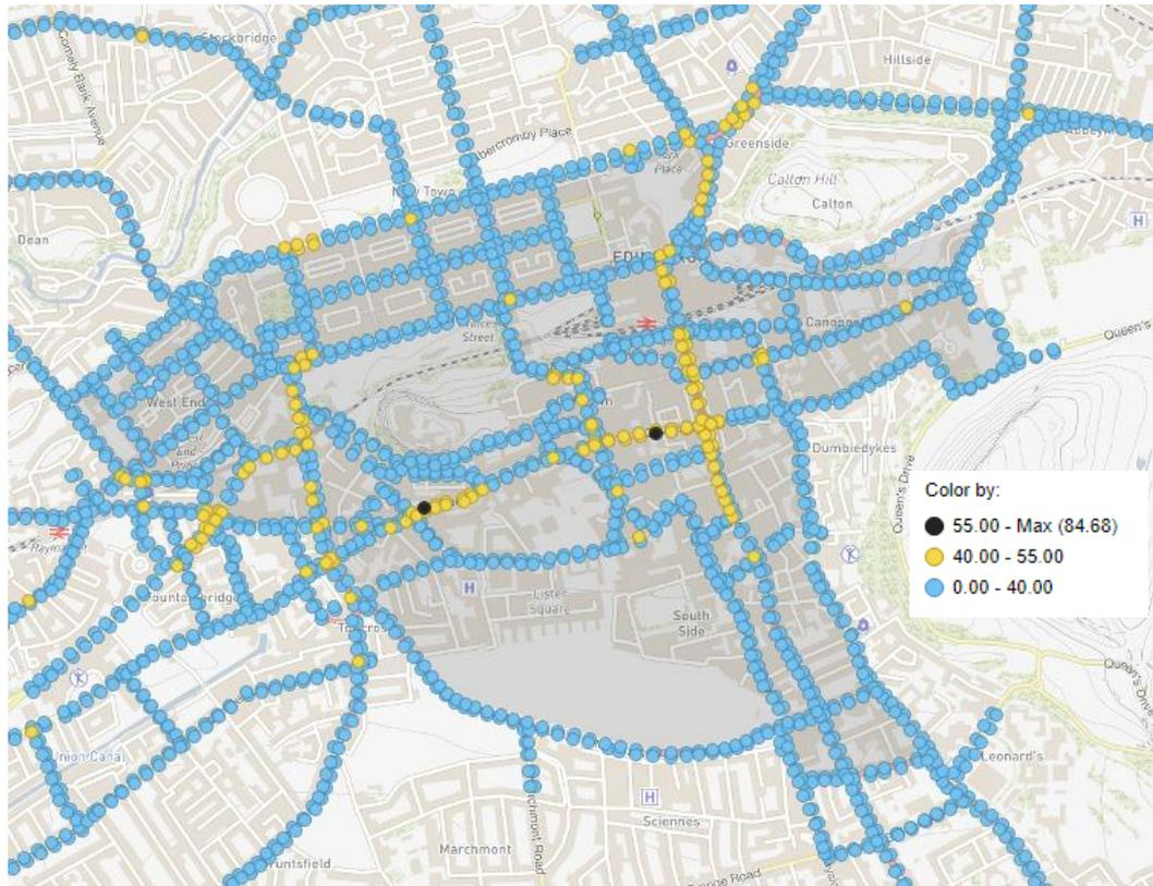
Figure 56: Base 2023 'future' scenario NO<sub>2</sub> predicted concentrations ( $\mu\text{g m}^{-3}$ )
