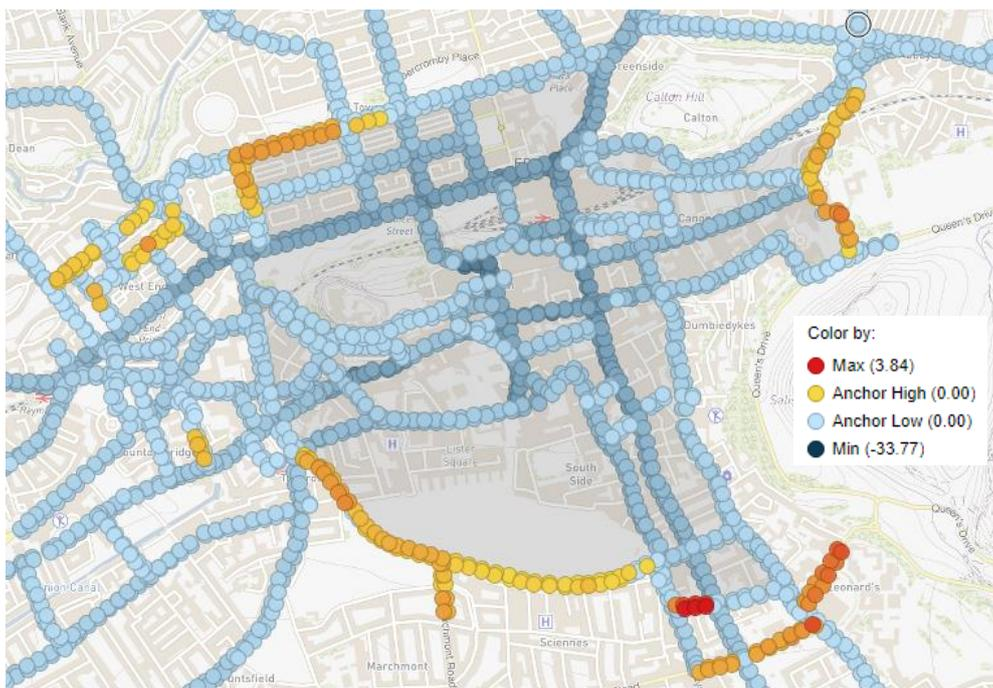
Figure 49: Predicted Changes in NO<sub>2</sub> concentration ( $\mu\text{g m}^{-3}$ ) due to introduction of Small LEZ (2019), when compared to Base 2019 scenario
