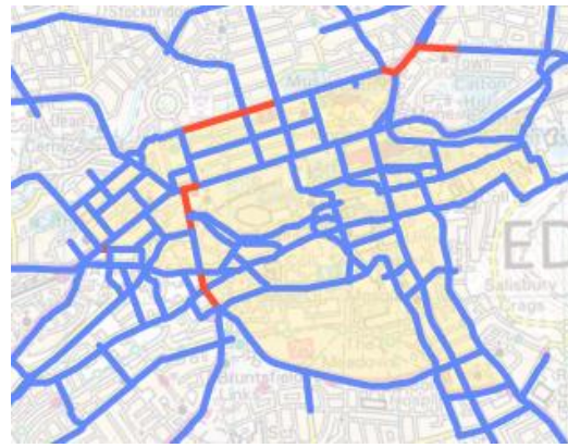
Figure 21: Large LEZ Option (with CCT) NO x Emission Rates 2023 (g/km/s) (Yellow Zone is Large LEZ)
