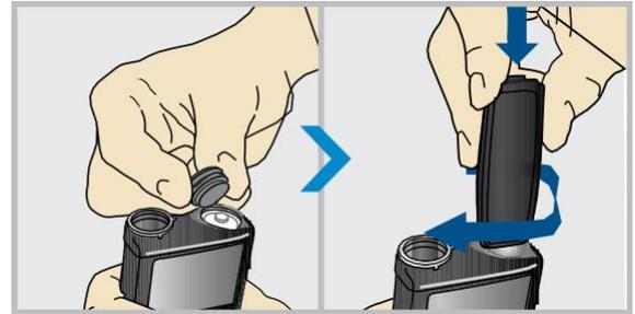
3. Place battery cap into the pump and use the edge of the belt clip to screw the cap back on.
