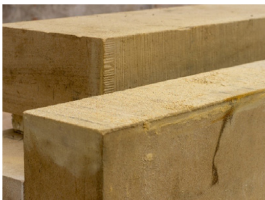
Sandstone blocks for stone repair.
