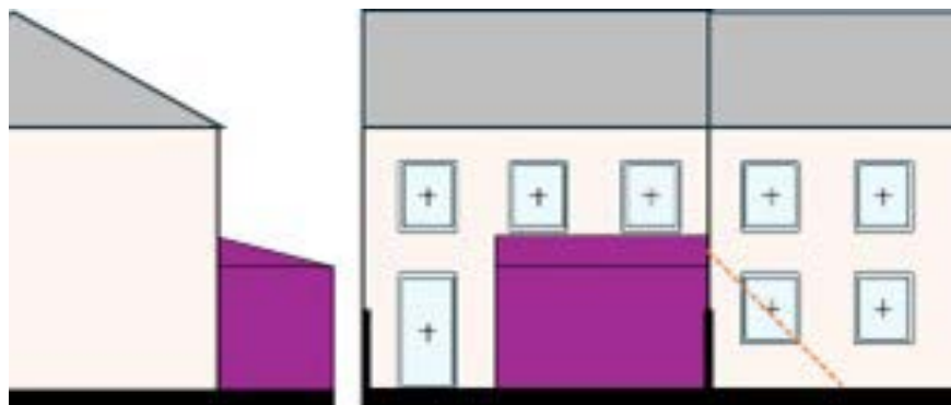
Mono pitched roof test taken from halfway point
