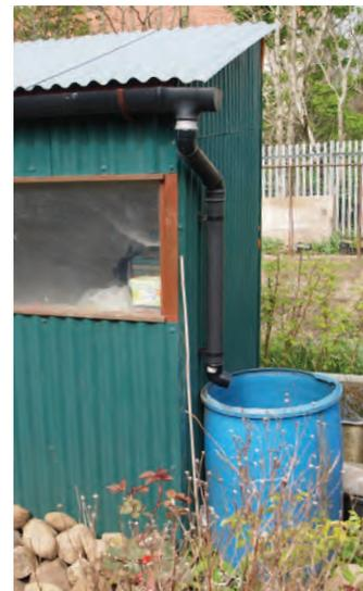
A DIY water butt collects the water from a plastic gutter. The single pitch of the hut minimises infrastructure. Mansewood, Glasgow
