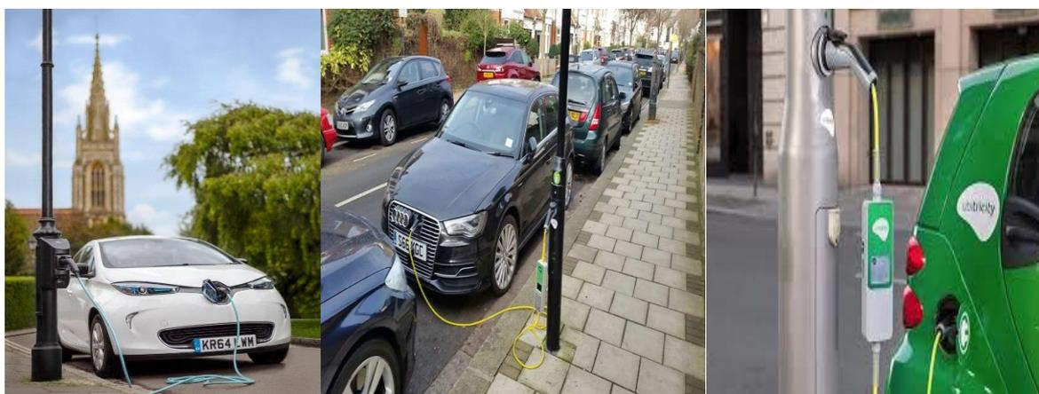
Figure 1: Examples of Lamppost Charging for EVs
