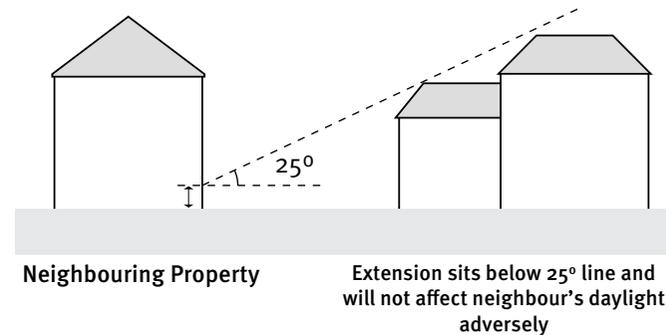
For rear extensions on terraced or semi-detached houses, adequate daylight will be maintained to the neighbouring property if 45 degree lines drawn from the plan or section of the new extension do not enclose the centre of the neighbour's window.
